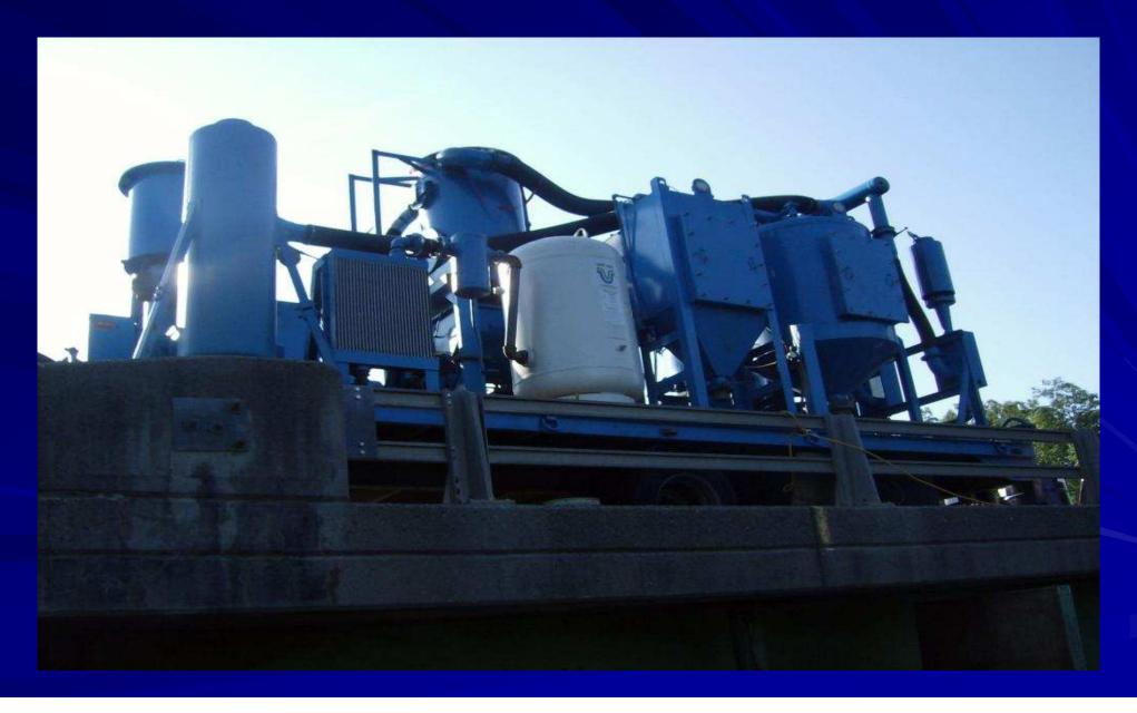
Classifier separates the lead flakes from the steel shot
